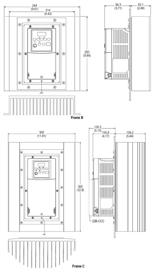
Figure B.4 PowerFlex 40 Flange Mount Drives – Dimensions are in millimeters and (inches)
