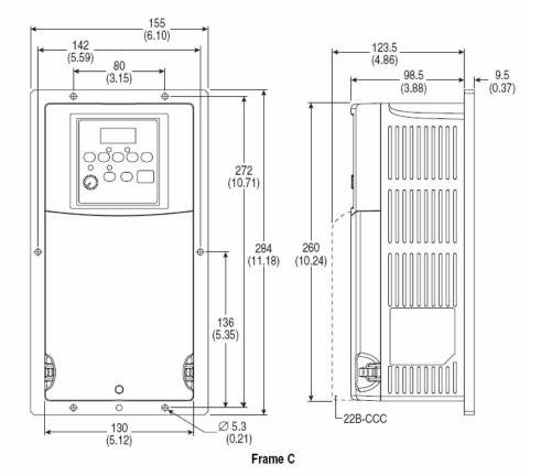
**Figure B.7 IP66, NEMA Type/UL Type 4X** – Dimensions are in millimeters and (inches) Weights are in kilograms and (pounds).
